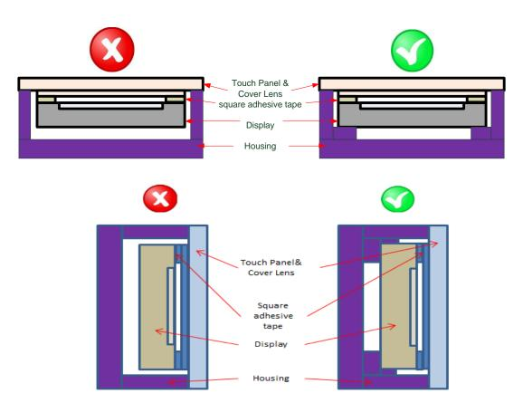
(6) TP needs to work in environment with stable stray capacitance. In order to minimize the variation in stray capacitance, all conductive mechanical parts must not be floating. Intermittent floating any conductive part around the touch sensor may cause significant stray capacitance change and abnormal touch function. It is recommended to keep all conductive parts having same electrical potential as the GND of the touch controller module.
