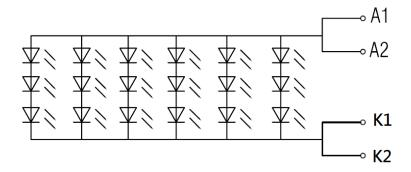
Note(6) When LCM is operated over 60°C ambient temperature, the IAK of the LED backlight should be adjusted to 150mA max
