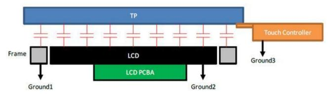
GND1, GND2 and GND3 should be connected together to have the same ground
