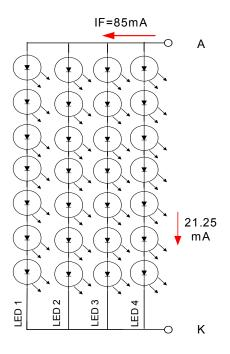
Note 3 When LCM is operated over  $40^{\circ}$ C ambient temperature, the IF should be follow :
