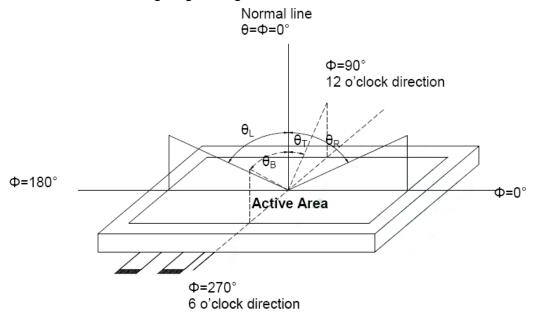
Note 2 Definition of optical measurement system
