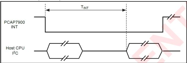
Report rate = 1 / TINT, it depends on properties of touch screen such as resistive value, I2C clock rate, channel number, thickness and material of cover lens, etc. For better touch performance, we strongly recommend using the 400K clock rate.
