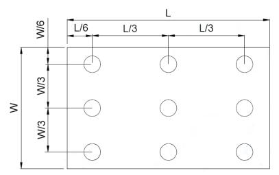
B<sub>max</sub>: The measured maximum luminance of all measurement position.
