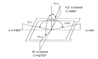
Note1: Definition of Viewing Angle: The viewing angle range that the CR>10
